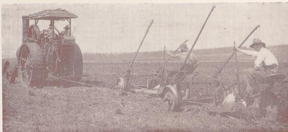
Steam ploughing is coming into vogue in Natal. The above illustrates the "direct traction" method
